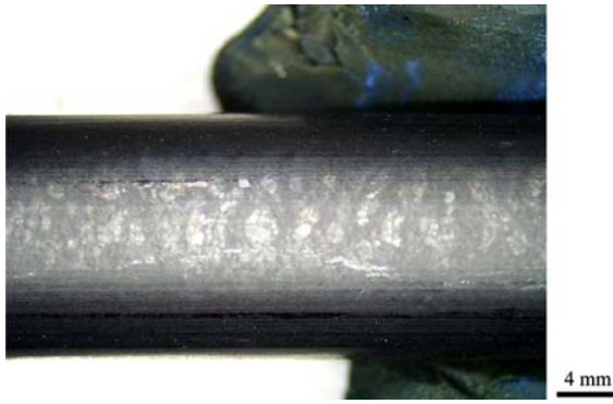
Fig. 1 A typical phosphated specimen with network defects (Phosphated layer was removed by mechanical polishing)
